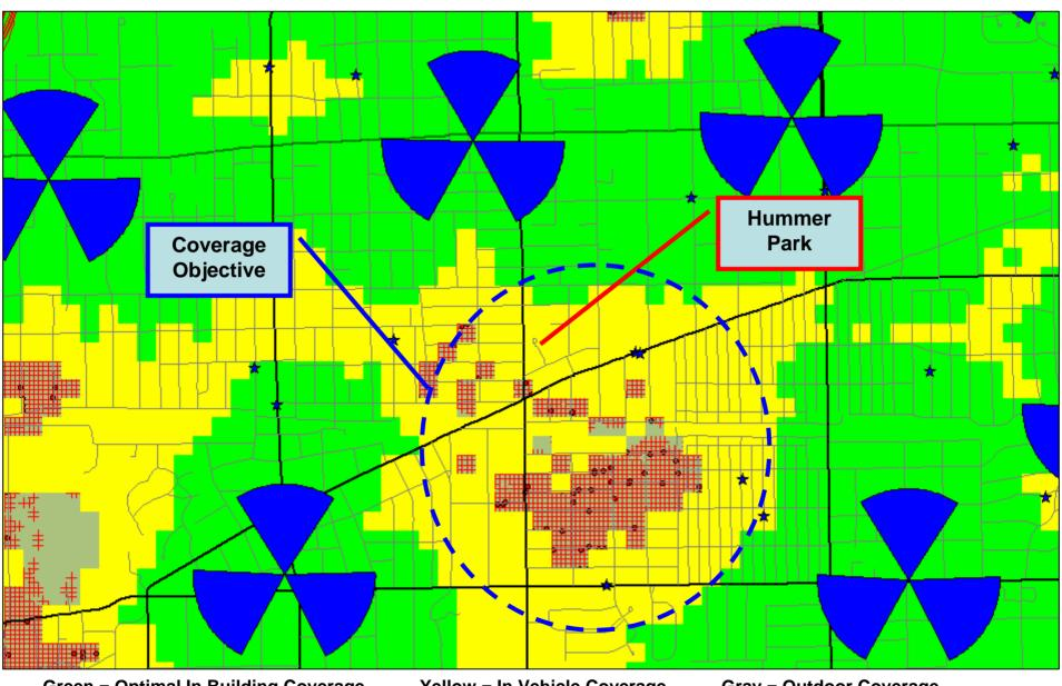
Green = Optimal In Building Coverage Red = Poorly Covered Residential Yellow = In Vehicle Coverage
