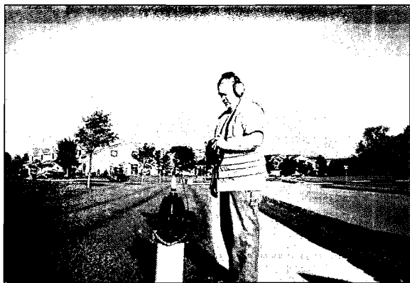
Conducting initial listening survey
