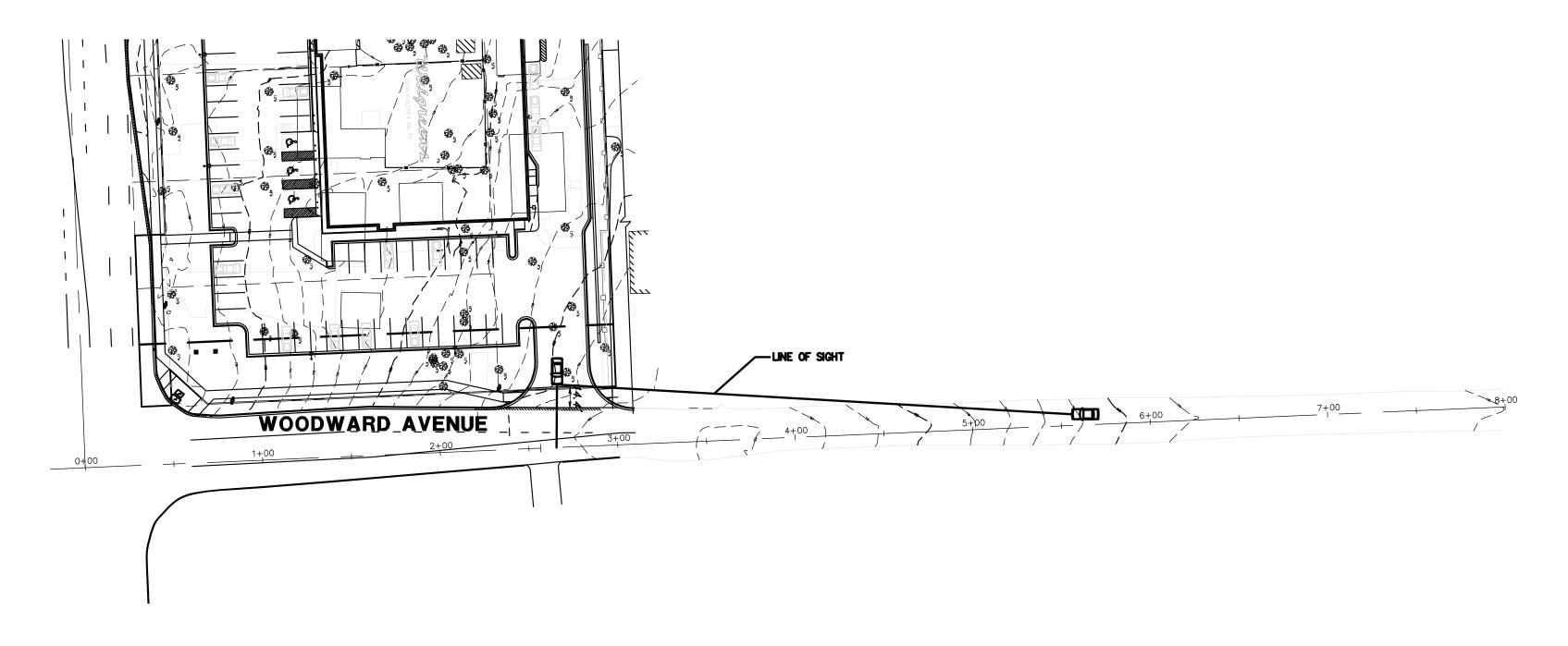
POSTED SPEED LIMIT ON WOODWARD AVENUE = 25 mph DESIGN SPEED ON WOODWARD AVENUE = 30 mph SLOPE OF WOODWARD AVENUE = 4.8% REQUIRED STOPPING SIGHT DISTANCE = 190 feet ACTUAL STOPPING SIGHT DISTANCE = 290 feet
