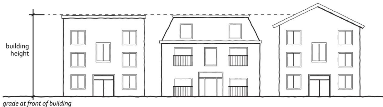
Figure 14-15: Generally Applicable Building Height Measurement
