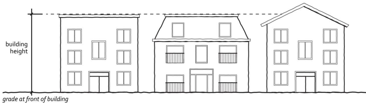
Figure 14-15: Generally Applicable Building Height Measurement
