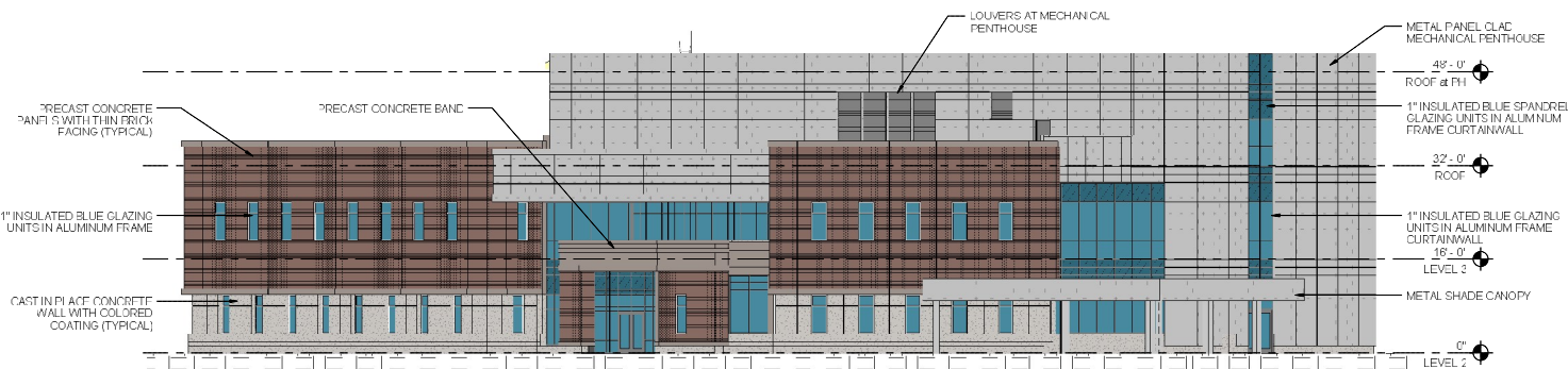
2 BUILDING ELEVATION WEST 3/32" = 1'-0"
