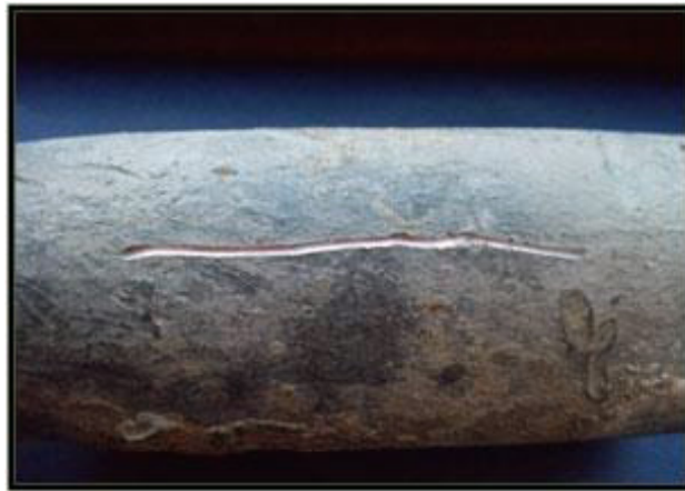
A lead pipe can be easily scratched with a key
