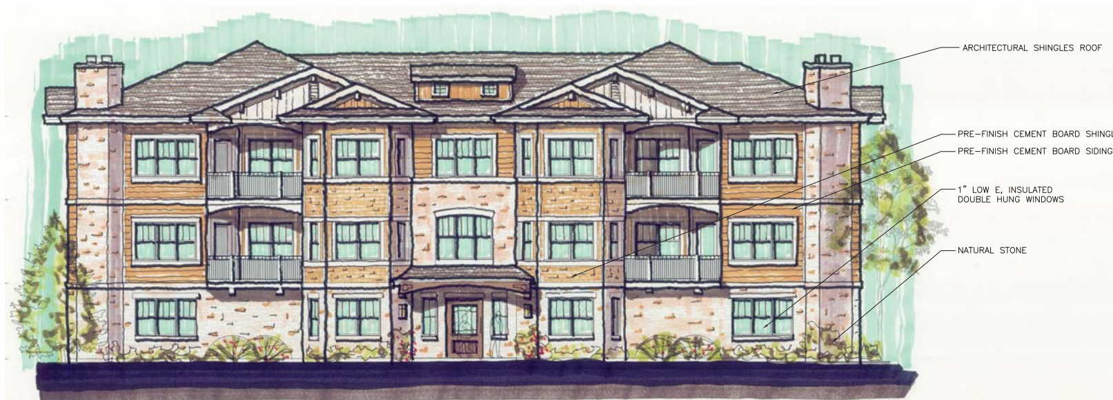
1 CONCEPTUAL ENTRY ELEVATION SCALE: 1/8"=1'-0"
