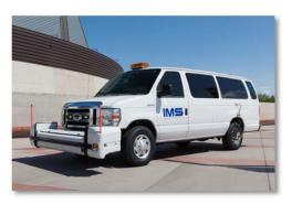
recommended for use on divided streets and arterials and collectors with four or more lanes of traffic. The surface condition survey is conducted continuously over the entire length of the test section and is not based on sample sections. The information gathered in this survey includes inventory, roughness, rut depth, cracking, and texture. The effects of environmental conditions will be considered in conjunction with the surface condition.
