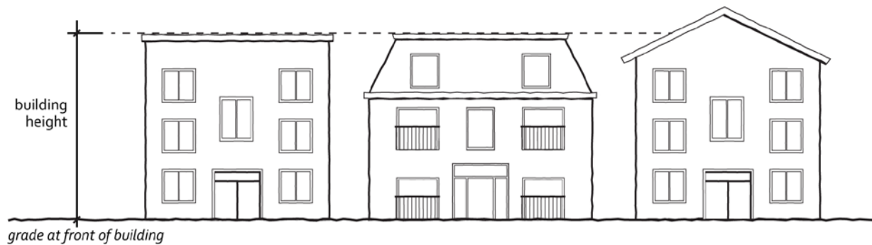
Figure 14-15: Generally Applicable Building Height Measurement
