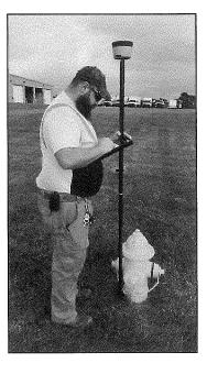
field teams utilize Trimble® R2 units for sub-foot accuracy. The level of accuracy taken will be based upon the above scope of work.
