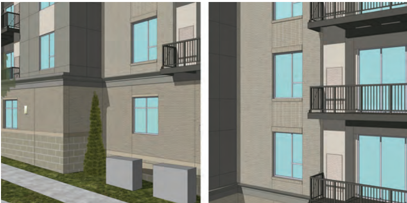
Material Details Special attention is paid to the details of the materials. A waterable detail is included to anchor the building to the ground, separating a strong limestone-style block proportion from the pedestrian scaled brick pattern above. The seams are thoughtfully laid out, windows and light fixtures respond accordingly. A spandrel detail is used throughout the project, shown here on the right with a different brick pattern plus a classic window head and sill detail. The unique balconies on Maple add an additional level of detail and sophistication.
