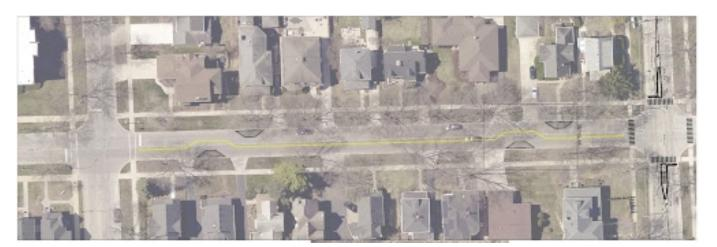
This is the option originally presented by staff, and remains the preferred approach. Two pairs of chicanes would be constructed as shown in the image, with centerline striping used for the entire block to define the travel lanes in each direction and provide visual lane narrowing. White parking box striping would be used to define the parking areas and support the lane narrowing effect for southbound traffic when no vehicles are parked there.
