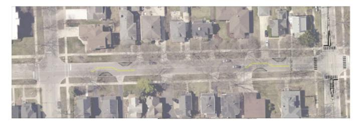
This option would be similar to that above, however centerline striping would only be used through the chicanes. Parking box striping would not be used with this option.
