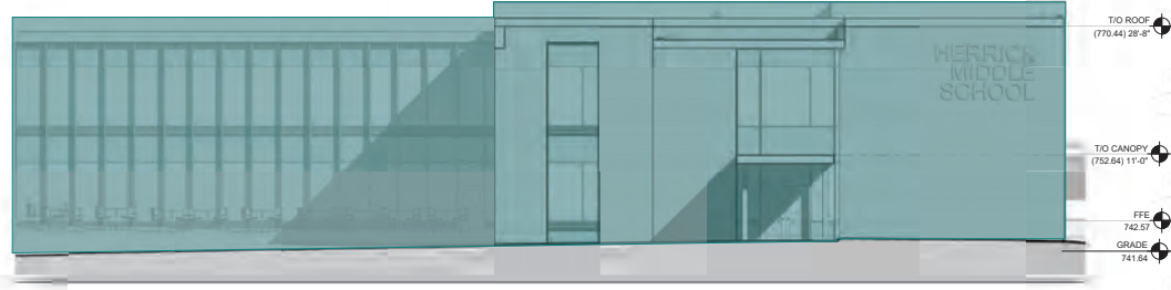
③ ELEVATION - EAST (CLASSROOMS) SCALE: 1/8" = 1'-0" TO ROOF (770.44) 28'-8" TO CANOPY (752.64) 11'-0" FFE 742.57 GRADE 741.64
