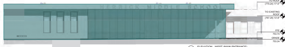
① ELEVATION - WEST (MAIN ENTRANCE) SCALE: 1/8" = 1'-0" TO ROOF (770.24) 17'-0" EXISTING ROOF (767.29) 13'-8" FFE 753.74 GRADE 753.24
