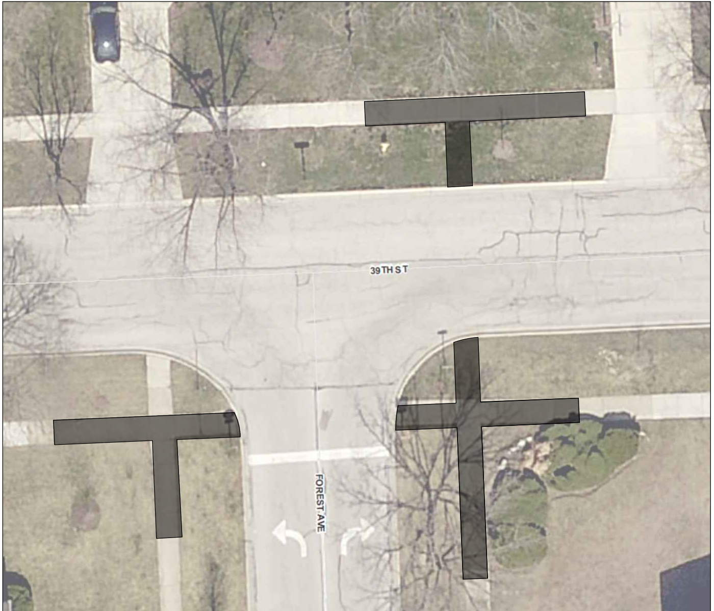
39th St and Forest Ave: Remove Ramp on Southwest corner and restore with topsoil and sod, Excavate and install new North-South crossing on East side
