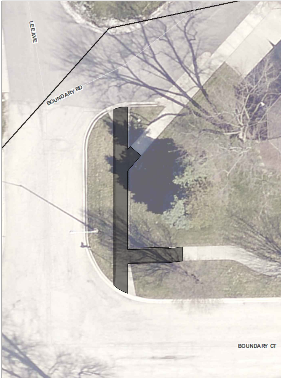
Boundary Ct and Lee Ave: Excavate for ADA Compliance, Install Concrete Curb Type B
