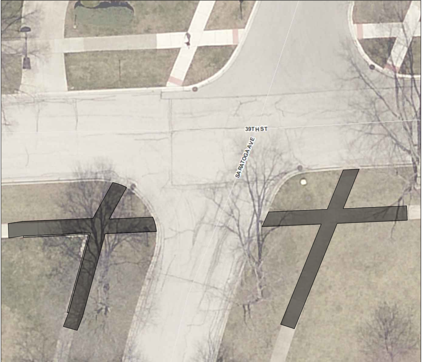
39th St and Saratoga Ave: Excavate and install Concrete Curb Type B on Southwest corner for ADA Compliance
