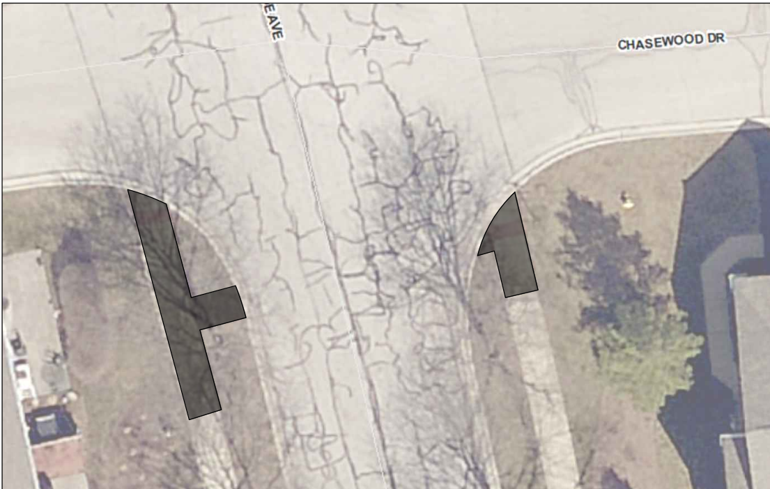
Chase Ave and Chasewood Dr: Excavate and install new East-West crossing
