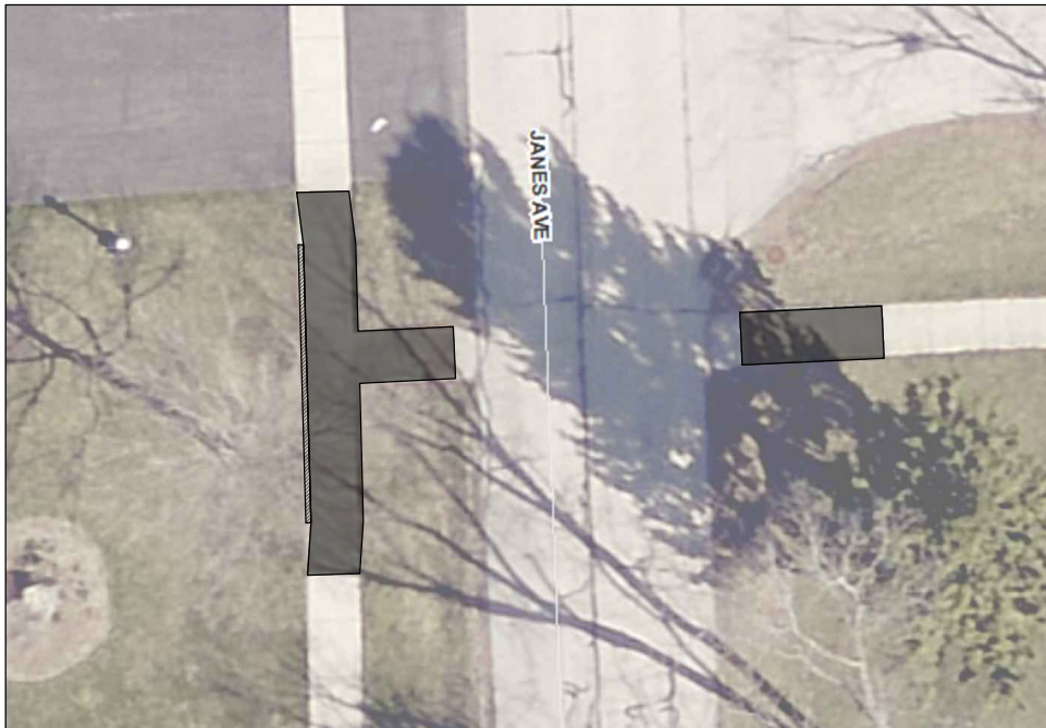
Janes Ave and 62nd St: Excavate west side for ADA Compliance, install Concrete Curb Type B
