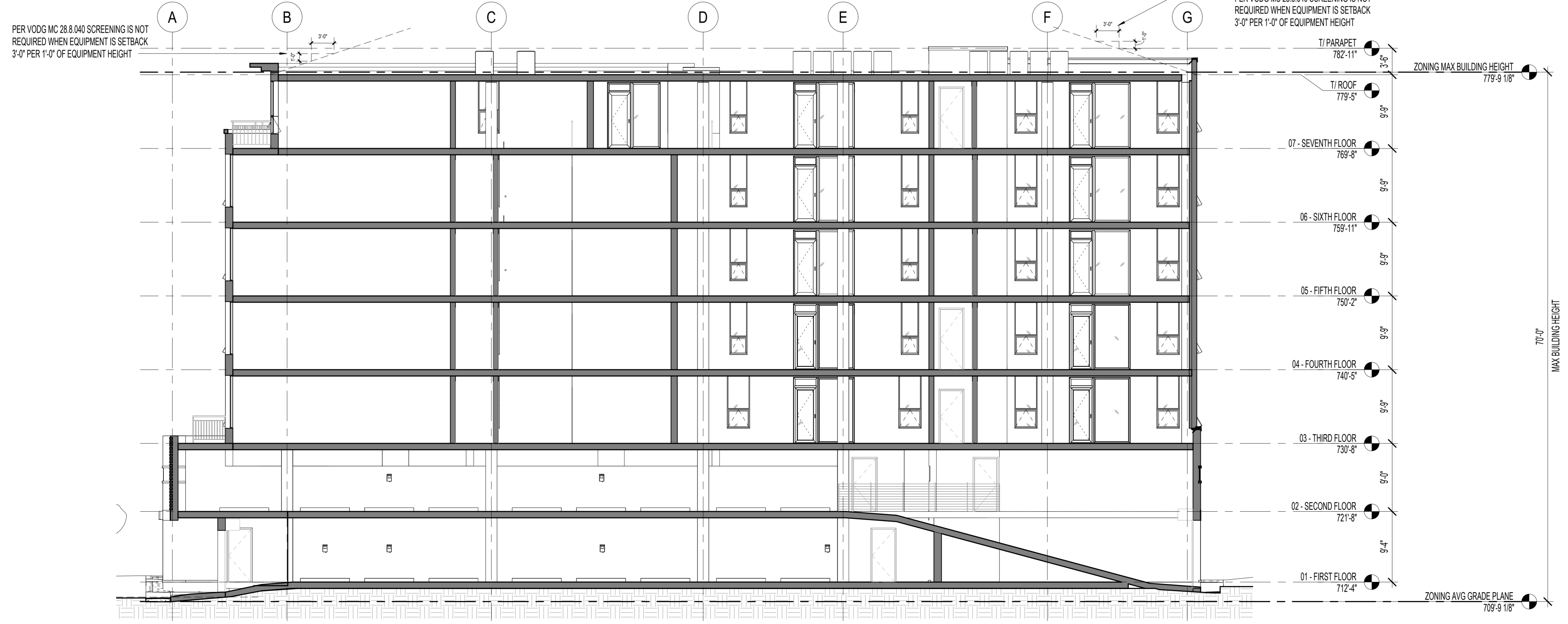
1 BUILDING SECTION THROUGH PARKING GARAGE RAMPS SCALE: 1/8" = 1'-0"
