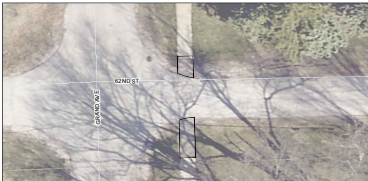
Grand Ave and 62nd St: HMA Pavement Removal to replace with PCC Sidewalk with HMA Transition and Detectable Warnings
