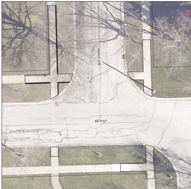
Osage Ave and 60th St: Lower Northwest Corner ramp for ADA Compliance (excavation approximately 4.5" with side curb), R&R other corners
