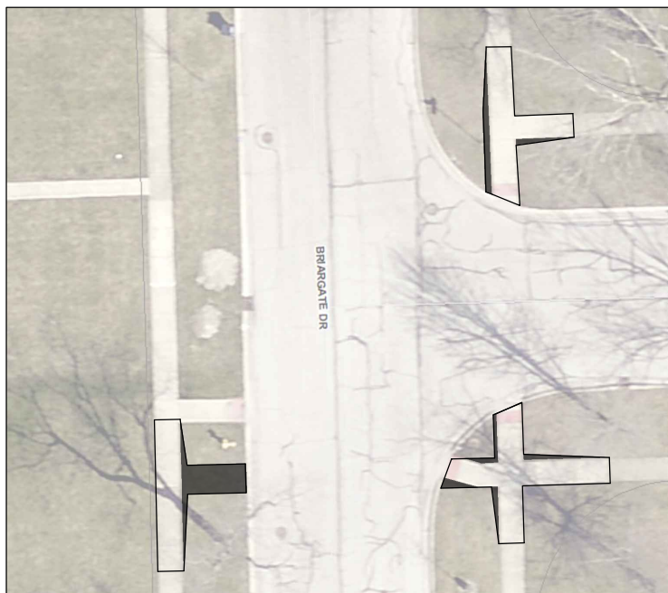
Briargate Dr and 66th St: Move E-W ramp at southwest corner south, Align E-W ramp at southeast corners, Widen ramps and keystones to 5' width, and Add transitions from from 5' width to existing 4' width
