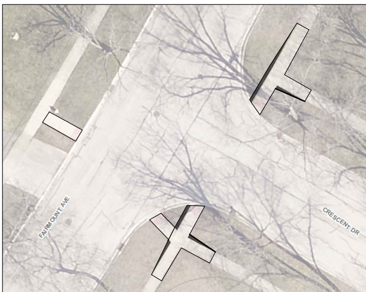
Fairmount Ave and Crescent Dr: Remove E-W ramps at southwest and southeast corners, Widen keystones to 5' width, and Add transitions from from 5' width to existing 4' width
