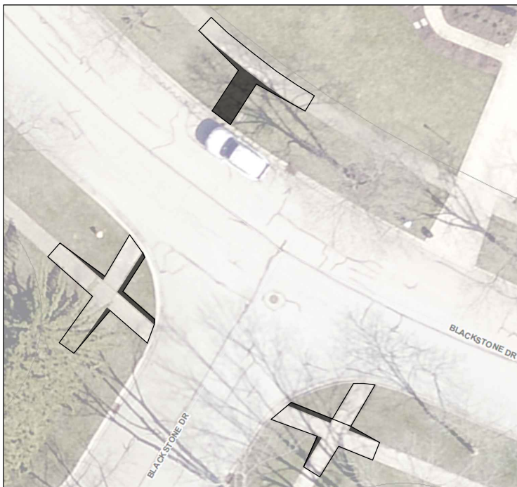
Blackstone Dr and Blackstone Cul de Sac: Add N-S ramp at northwest corner, Remove N-S ramp at southeast corner, Widen ramps and keystones to 5' width, and Add transitions from from 5' width to existing 4' width
