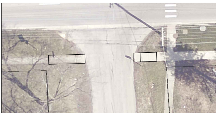
Fairmount Ave and 63rd St: PCC Sidewalk removal, replace with PCC Sidewalk and HMA transition at road edge
