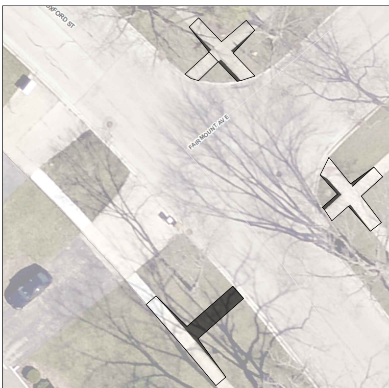
Oxford St and Fairmount Ave: Remove NE-SW ramp at northeast corner, Add NE-SW ramp at southwest corner, Widen ramps and keystones to 5' width, Add transitions from from 5' width to existing 4' width.
