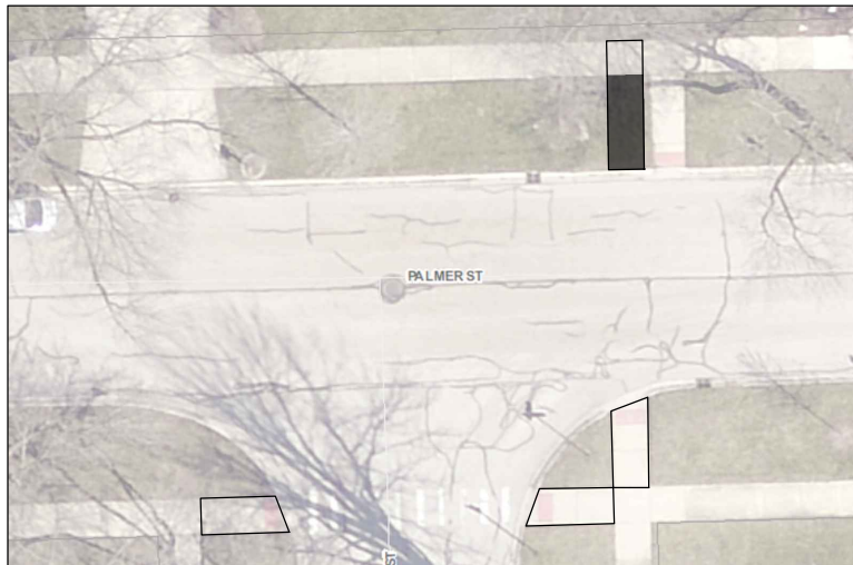
Palmer St and Powell St (South Leg): Realign northeast corner N-S ramp. R&R other corners as shown.
