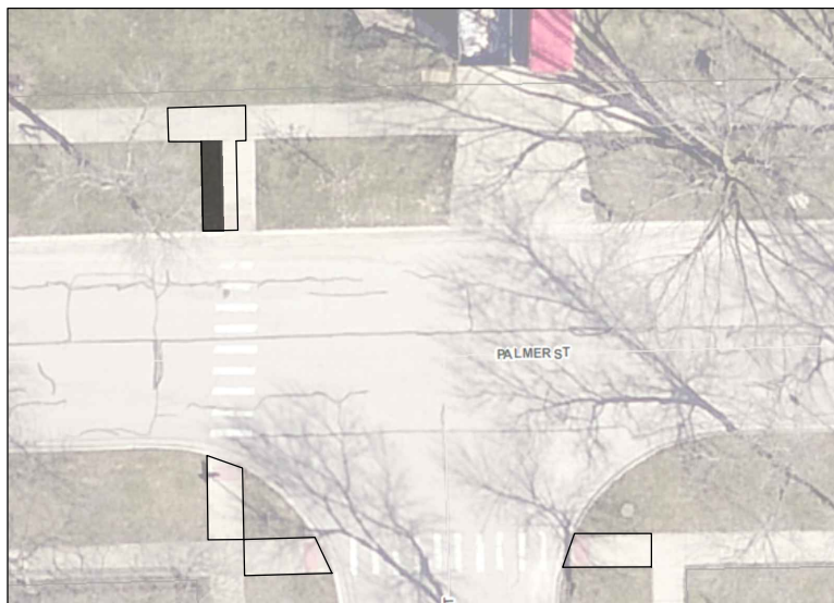
Palmer St and Barrett St: Realign northwest corner N-S ramp. R&R other corners as shown.
