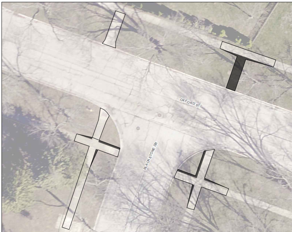
Oxford St and Blackstone Dr: Remove northwest ramp and southwest N-S ramp, Add northeast N-S ramp, Widen ramps and keystones to 5' width, and Add transitions from from 5' width to existing 4' width
