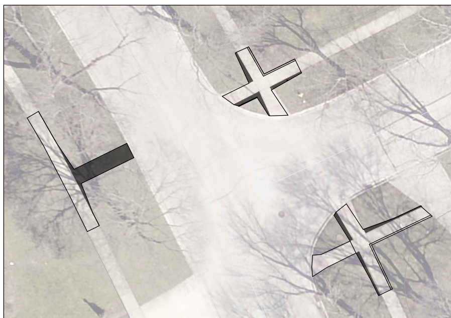
Fairmount Av & 67th St (East Leg): Add E-W ramp at northwest corner, Lower northeast keystone for ADA Compliance (excavation approx 2" with side curb), Remove Ramp at southeast corner and lower keystone for ADA Compliance (excavation approx 4" with side curb), Widen ramps and keystones to 5' width, and Add transitions from from 5' width to existing 4' width
