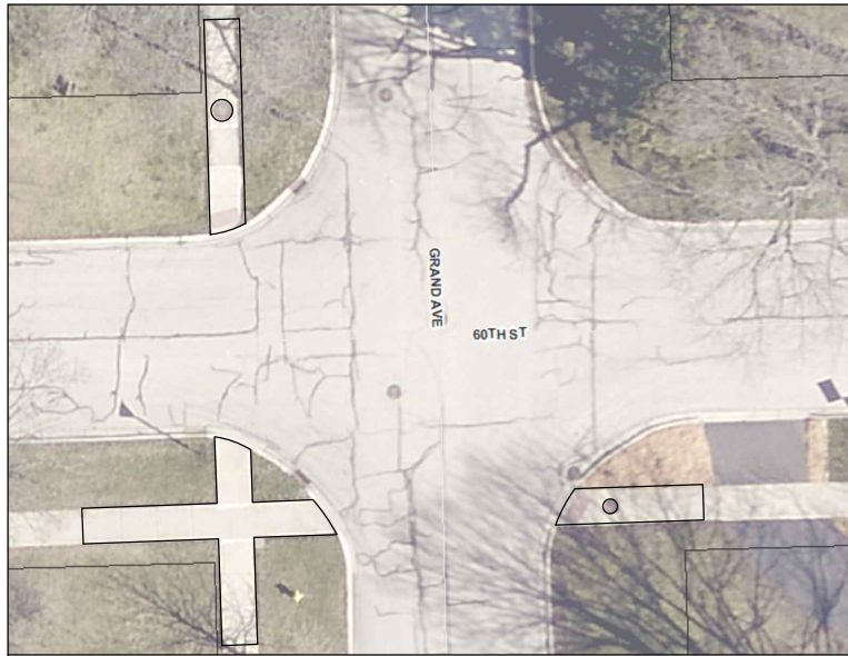
Grand Ave and 60th St: Lower Northwest Corner ramp for ADA Compliance (excavation approximately 3"), adjust manholes, R&R other corners
