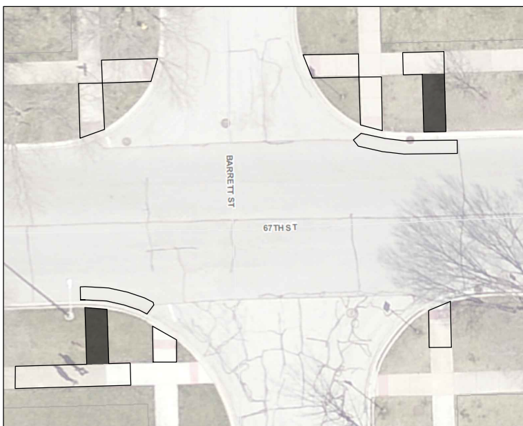
Barrett St and 67th St: Shift N-S ramp at southwest corner west, Shift N-S ramp at northeast corner east. Patch street as necessary. R&R other corners as shown.
