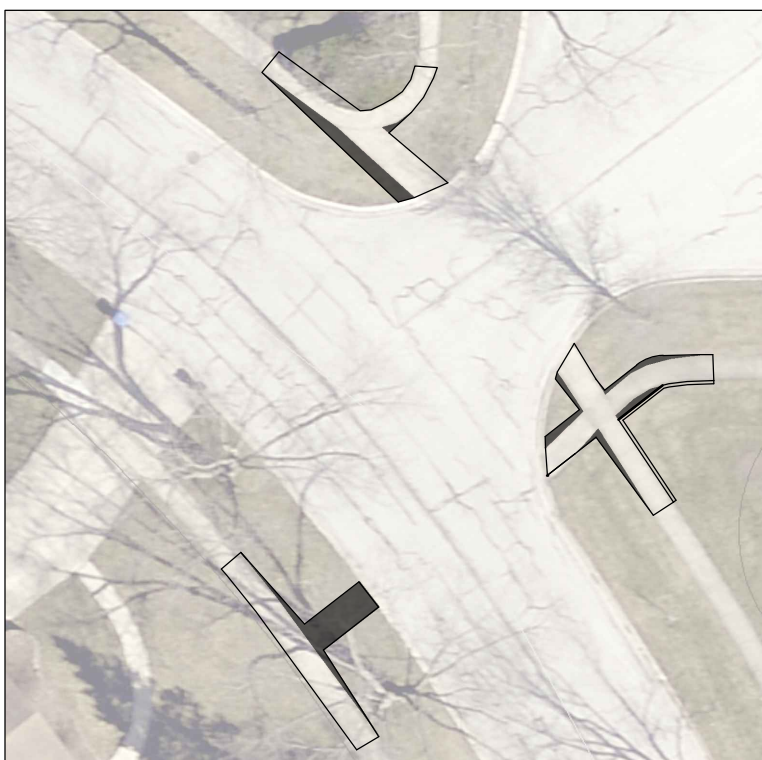
Briargate Dr and Briargate Cul de Sac: Add NE-SW ramp at southwest corner, Lower southeast corner keystone for ADA Compliance (excavation approx 7" with side curb), Widen ramps and keystones to 5' width, Add transitions from from 5' width to existing 4' width.
