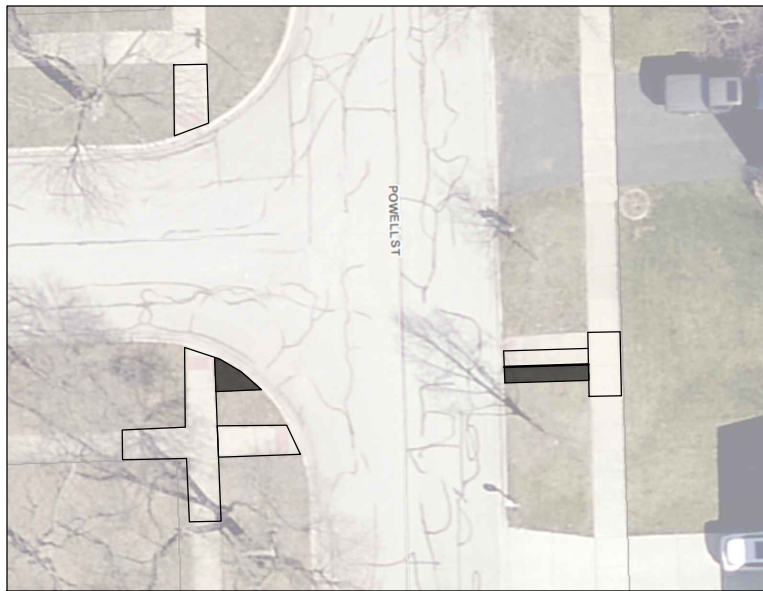
Powell St and Saylor St: Shift E-W ramps at southeast and southwest corners to align. R&R other corners as shown.
