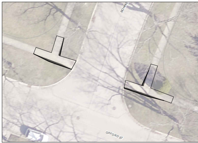
Oxford St and Bonnie Brae Dr: Widen ramps and keystone to 5' width, transition from from 5' width to existing 4' width
