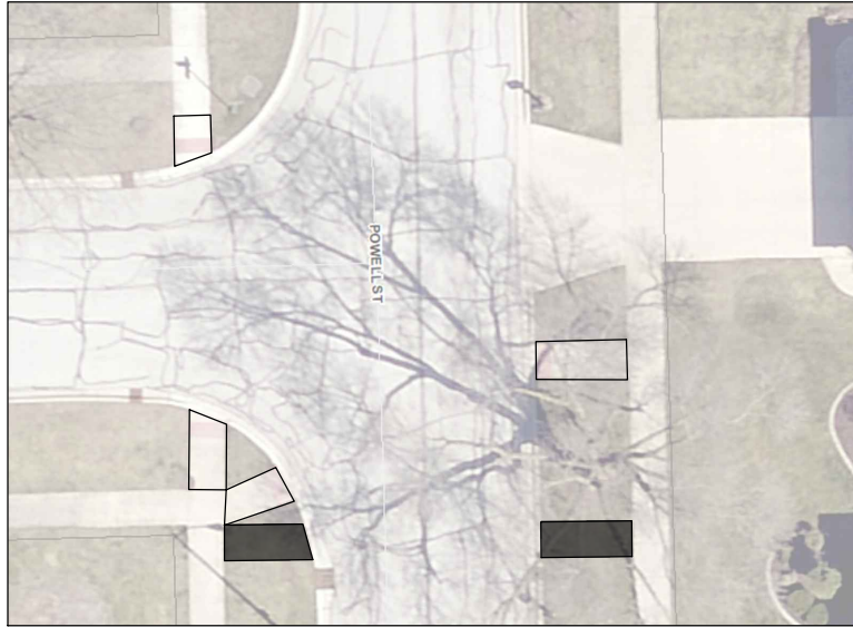
Powell St and 67th Pl: Shift E-W ramp at southwest corner south, Shift E-W ramp at southeast corner south to align. R&R other corners as shown.
