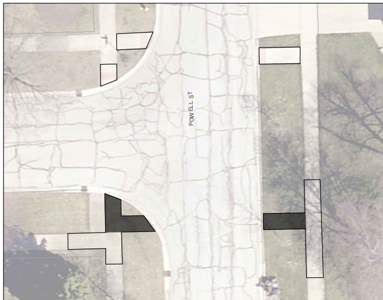
Powell St and 68th Pl: Remove E-W ramps at northwest and northeast corners. Shift N-S ramp at southwest corner east. Add E-W ramps at southwest and southeast corners.
