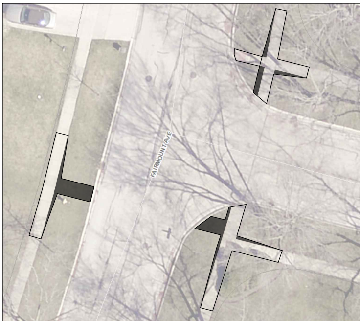
Fairmount Ave and Briargate Dr: Remove E-W ramp at northeast corner, Add E-W ramps to southwest and southeast corners, Widen ramps and keystones to 5' width, and Add transitions from from 5' width to existing 4' width
