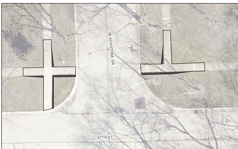
Blackstone Dr and 67th St: Widen ramps and keystones to 5' width, Add transitions from from 5' width to existing 4' width
