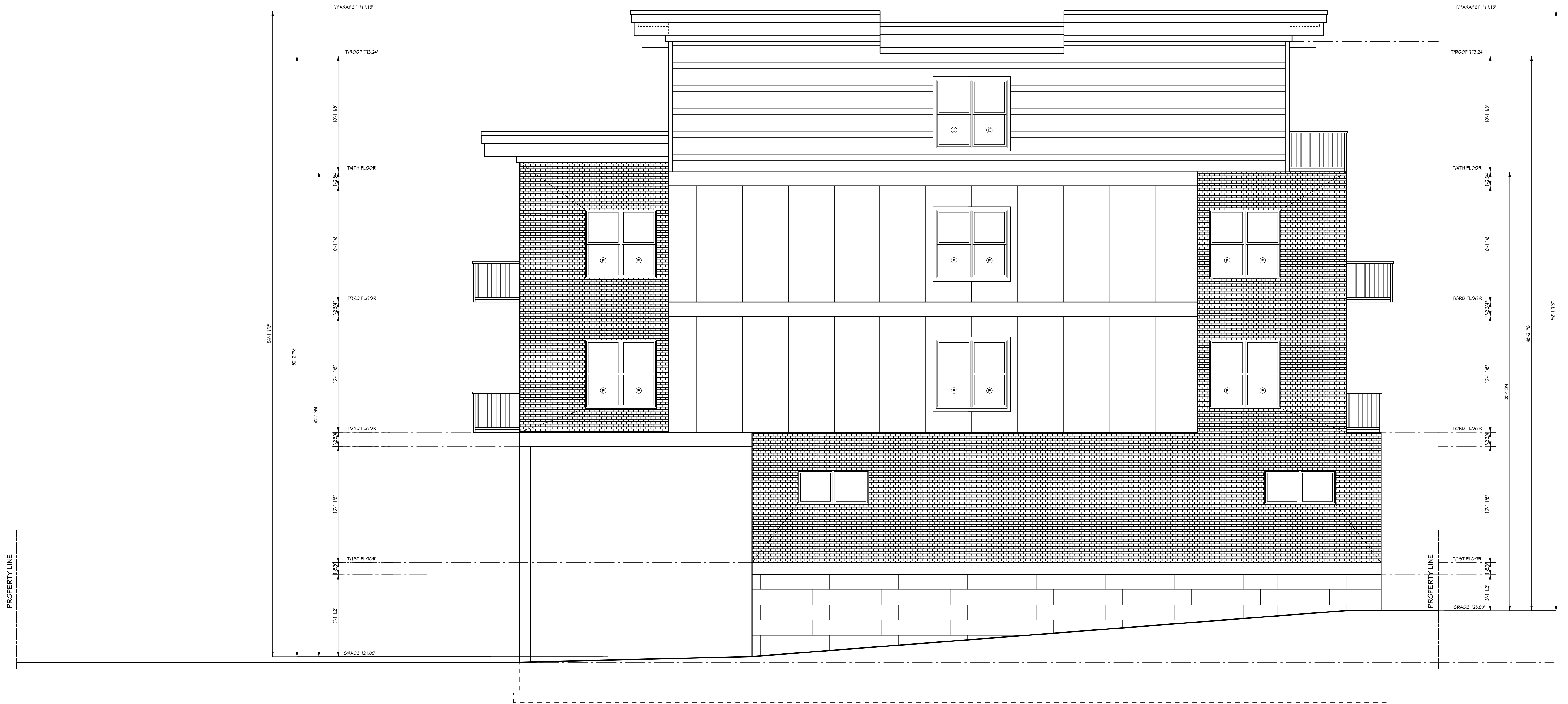
WEST ELEVATION SCALE: 1/4" = 1' 0" GLAZING AREA = 286 SF EXTERIOR WALL AREA = 3225 SF GLAZING = 8.9% OF WALL AREA
