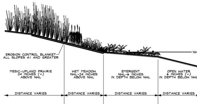
**NOT TO SCALE NATURALIZED STORMWATER BASIN SECTION**
