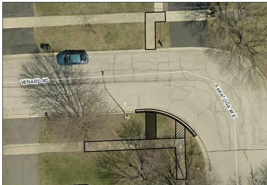
Southwest corner of Venard Rd & Saratoga Ave: Realign ramp. R&R other corner as shown.
