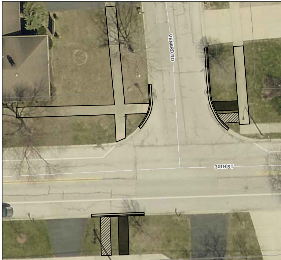
Venard Rd and 35th St: At Northeast corner, realign ramp. At southwest corner, realign ramp. R&R northwest corner as shown.
