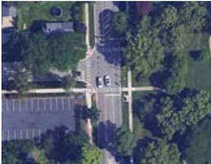
Piano key crosswalks at Fairview Avenue and Prairie Avenue
