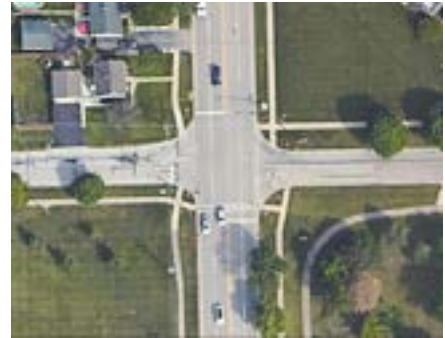
Piano key crosswalks at Fairview Avenue and Prairie Avenue
